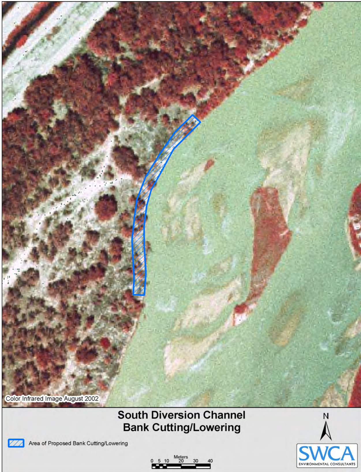
Figure 2.13. Example of the bank cutting/lowering technique.
